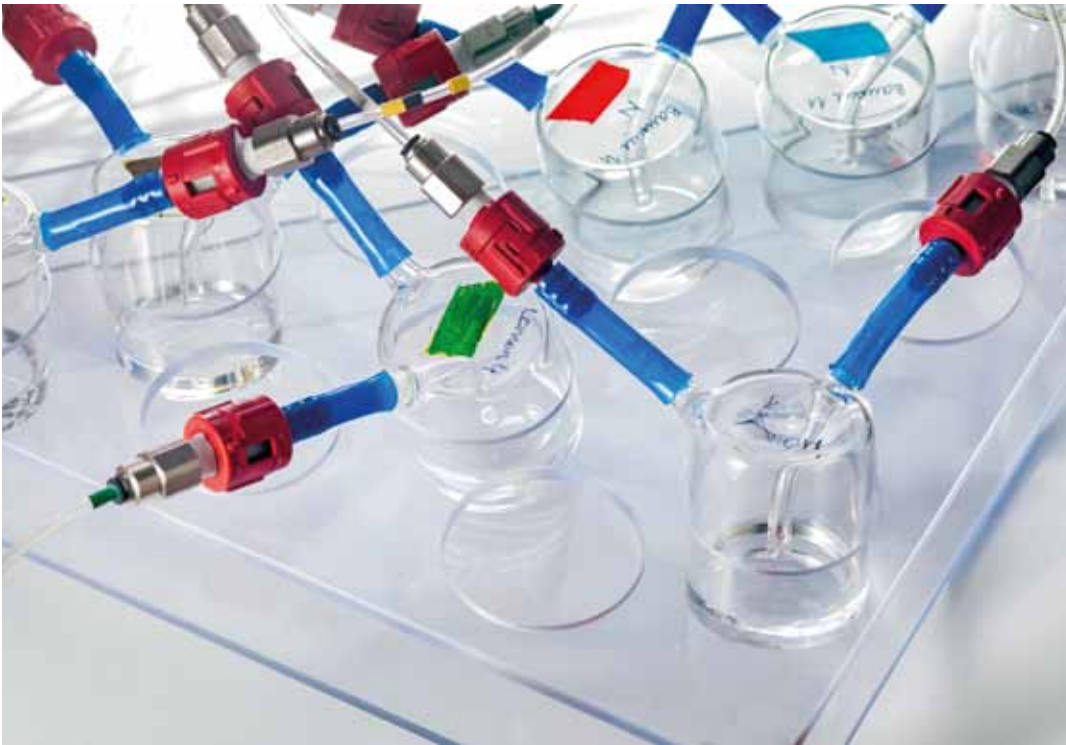
Figure 1: Smell plays a key role in food perception. To study smell and its interaction with other senses scientists use an olfactometer, a device to deliver odorants to human observers. Shown are jars with various odorants.
